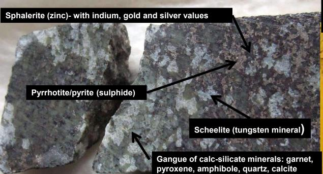
Mineralogy of a 400Kg bulk sample in 2016 by SGS Labs developed a **trial process mass balance with 75% recovery and 68% WO<sub>3</sub> concentrate using low-cost gravity methods.** Additional work is anticipated to finalize a flow sheet and include a potential zinc by-product.
